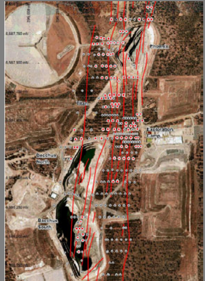
Drill plan showing location of QAQC & infill drilling in main resource areas & holes targeting high grade mineralisation in Bacchus Deeps area. Red filled collars are holes completed to date
